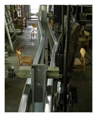
failure of the upper chord; interaction of bending and flexural buckling
