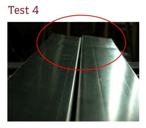
failure of a compression brace member; interaction of compression and bending
