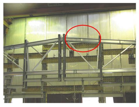
failure in the upper chord, interaction of bending (weak axis) and flexural buckling
