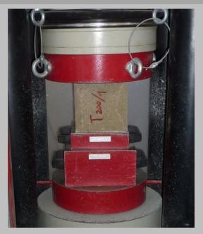
150 x 150 x 150 mm cubes 3-3 pieces in all heat step performed on the basis of the MSZ EN 12 390-3:2009 Standard
