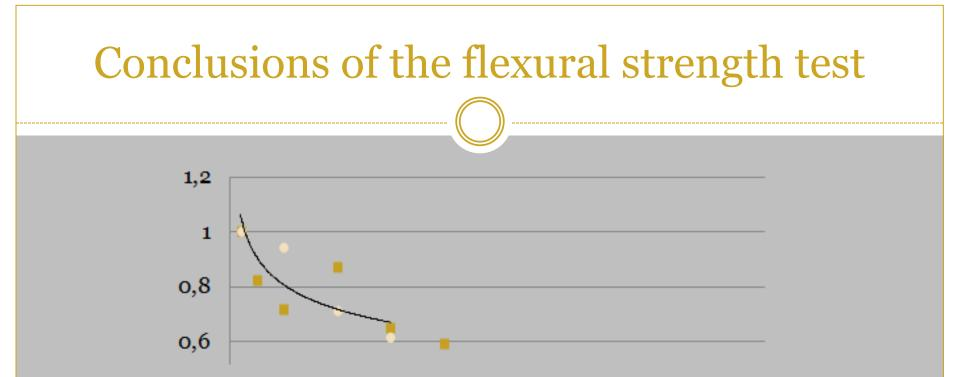
•the extent of the flexural strength reduction of polymer concrete is higher than the extent of compressive strength reduction;
