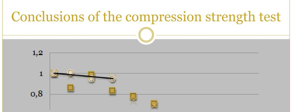
• the extent of the strength reduction of polymer concrete does not exceed the strength reduction of concrete of the same strength, up to a heat load of 300°C;
