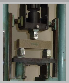
70 x 70 x 250 mm beams 3-3 pieces in all heat step performed on the basis of the MSZ EN 12 390-5:2009 Standard
