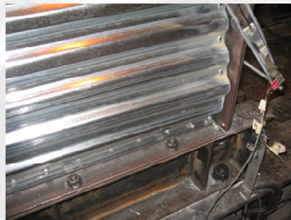
c) buckling and warping of corrugated sheet after screw pull-out
