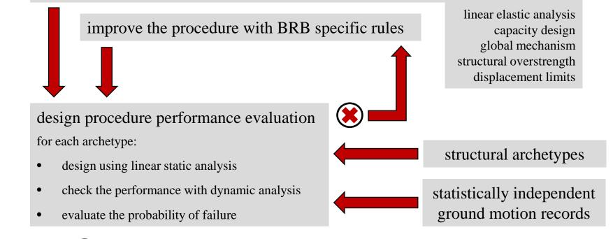
objective: develop a standardized BRBF design procedure
